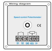
**S1-S2 Switch**: max.4A/250Vac. 10A/12Vdc **Control signal**: ADJ - GND 0-10V **U+ supply**: +10V /Max. 12Vdc / 1mA/
