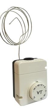
Frost protection thermostat is developed to protect ventilation components (water heaters) from freezing under cold weather and insufficient heating. Frost protection thermostat works under pressure of steam, reacts fast and has maximum sensitivity introducing external air.
